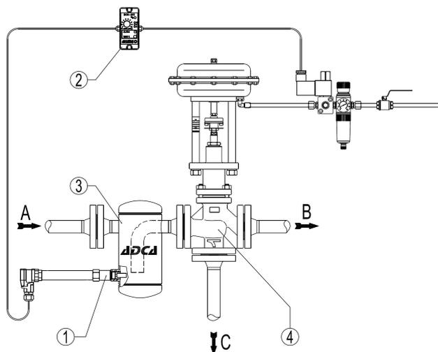
The BCS controller (2) is programmed to continuously measure (1) the electrical conductivity of boiler return condensate (closed related to the TDS) and, compare it with the set point selected in the controller, it will invert the flow of the three way valve (4) from B to C if the measured value is higher, or keep the valve flow from A to B until the measured value exceed the set point.
