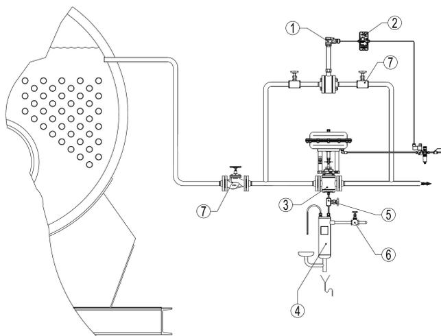
The VPC blowdown valve is programmed to open periodically in order to purge a certain amount of water. The BCS controller will then measure the electrical conductivity of boiler water (closed related to the TDS) and compare it with the set point selected in the controller. It close the valve after the purge if the measured value is lower, or it will keep the valve open until the measured value stay below the set point, if it is higher.
