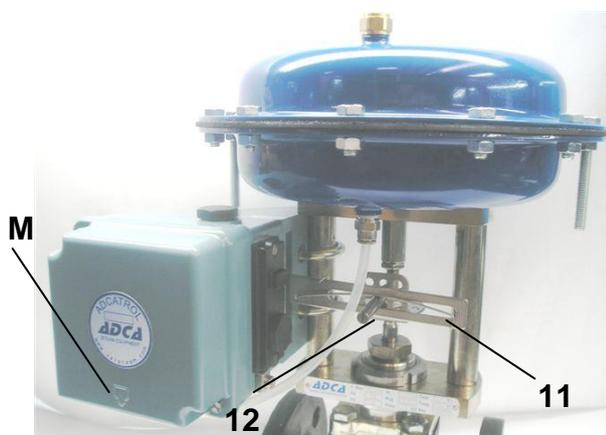
Ensure that the feedback lever **11** is horizontal at 50 % stroke.
