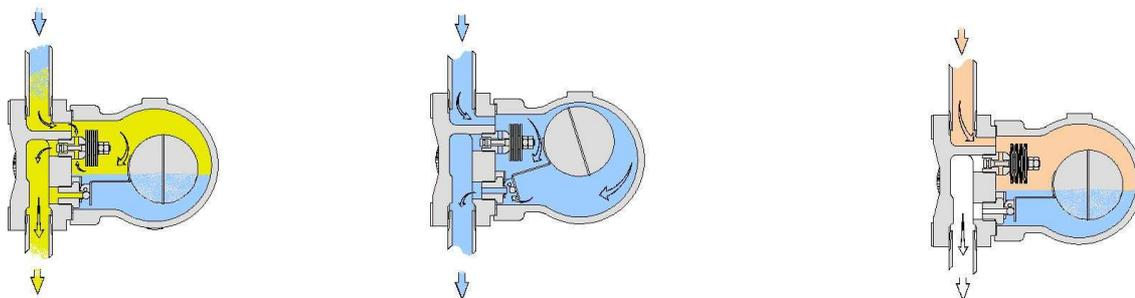
**THERMOSTATIC TRAPS BALANCED PRESSURE ( TH ) and BIMETALLIC ( BM )** operate on a difference in temperature between condensate and steam. They build up condensate so that its temperature drops down to a certain level below saturation temperature in order for the trap to open. By backing up condensate, the trap will tend to modulate open or closed depending on load.
