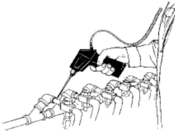
An ultrasonic test of steam traps is a positive test. The main advantage to ultrasonic testing is that it isolates the area being tested by eliminating confusing background noises. A user can quickly adjust to recognizing differences among various steam traps, of which there are three basic types: thermodynamic, mechanical and thermostatic (see Adca training Part 3).
