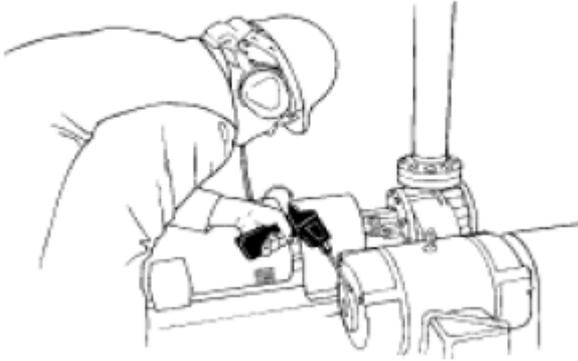
Ultrasonic inspection and monitoring of bearings is by far the most reliable method for detecting incipient bearing failure. The ultrasonic warning appears prior to a rise in temperature or an increase in low frequency vibration levels. Ultrasonic inspection of bearings is useful in recognizing:
