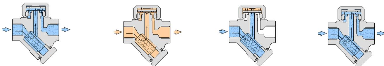
**INVERTED BUCKET ( IB )** traps usually fail in the open position because the trap loses its prime. This condition means a complete blow-through, not a partial loss. The trap will no longer operate intermittently. Aside from a continuous rushing sound, another clue for steam blow-through is the sound of the bucket clanging against the side of the trap.
