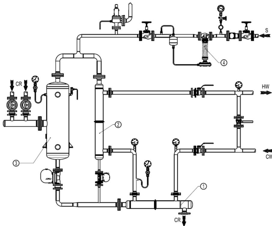
The condensate return (CR) is expanded on a flash vessel (3). The flash steam which is produced there and the remaining condensate are then directed to the respective heat exchangers (1 e 2) where in the meanwhile the pressurized feed water (CW) is heated (HW) before it passes to the economizer or be directly introduced into the steam boiler (it is recommended to install a by-pass from CW to HW).
